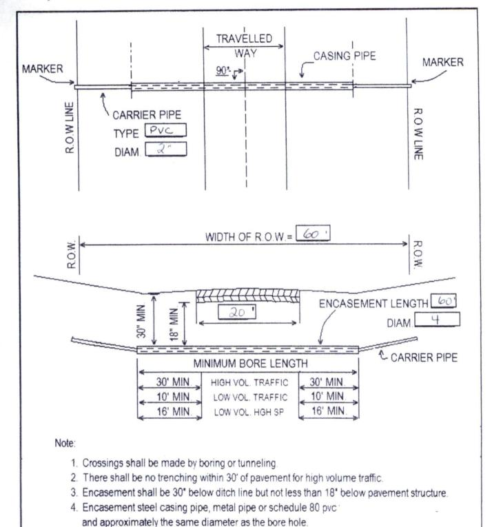
5. Line markers shall be placed at the R.O.W. line on both sides.
